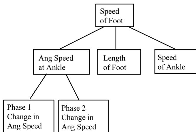
The speed of the ankle joint center immediately before impact is the sum of the linear speed of the center of the knee joint at that instant ( $v_k$ ) and the product of the angular speed at the knee ( $\omega_k$ ) and the length of the shank ( $l_s$ ), or:
