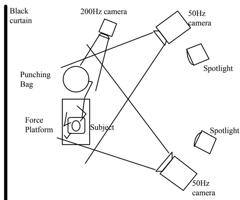
Figure 5. Overhead diagram of the data collection set-up.
