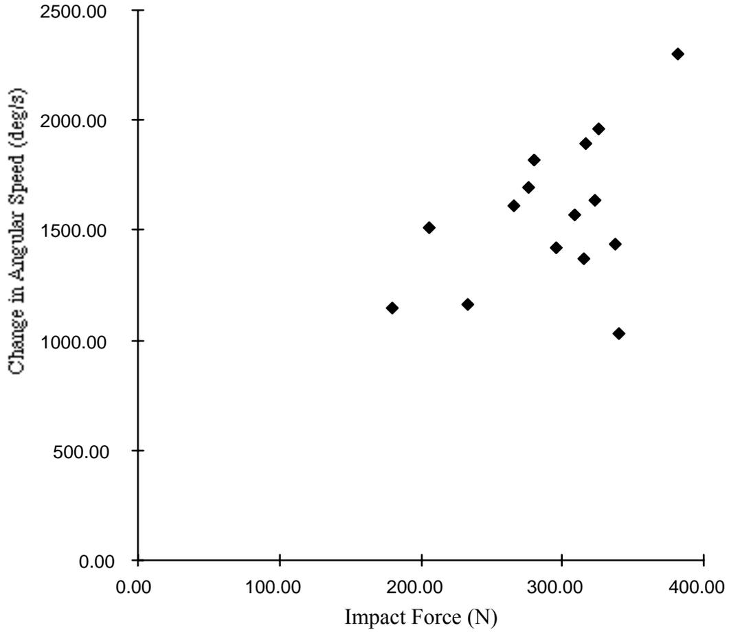
Figure F5. Plot of the change in angular velocity at the knee during Phase 2 against impact force.
