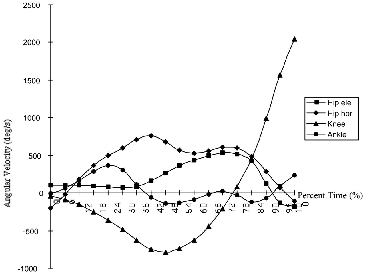
Figure 7. Average angular velocities at the joints of the kicking leg.
