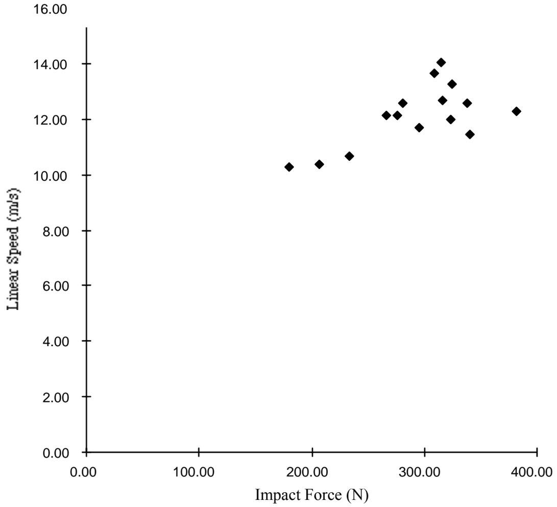
Figure F4. Plot of the linear speed of the ankle against impact force
