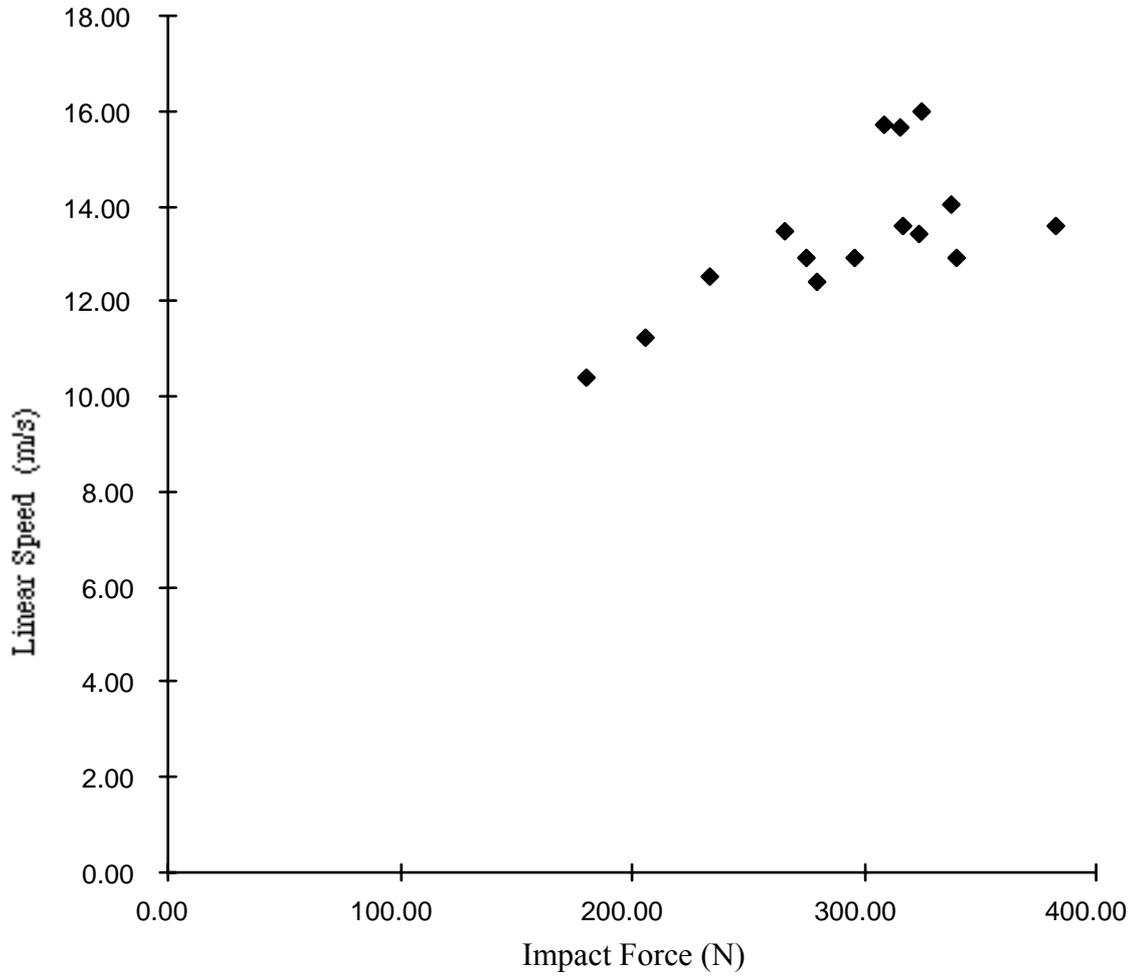
Figure F3. Plot of the linear speed of the toe against impact force
